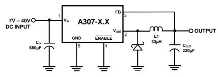
Figure 1. Fixed Output Voltage Versions
