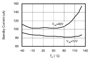
Standby Current vs. Input Voltage
