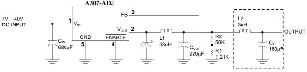
Figure 4. LC Filter for Low Output Ripple
