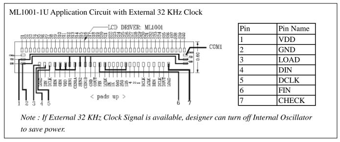
Note: Pin LOAD and Pin CHECK shall be connected together if the flip-chip assembly is in good condition. Hence, Pin CHECK can be served for qualifying the flip-chip assembly quality.
