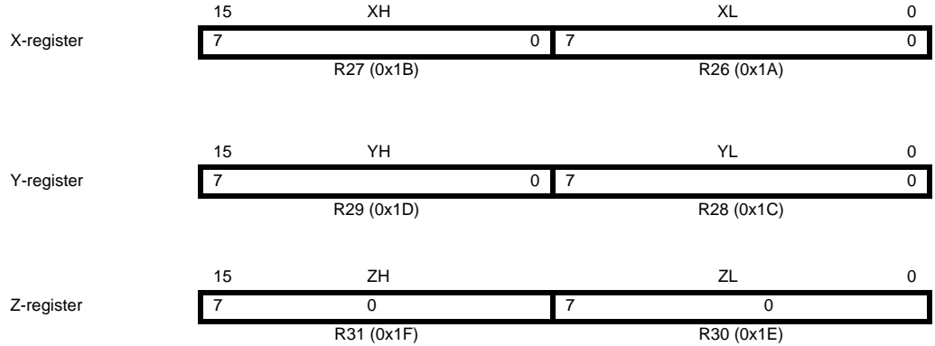
Figure 5. The X-, Y-, and Z-registers
