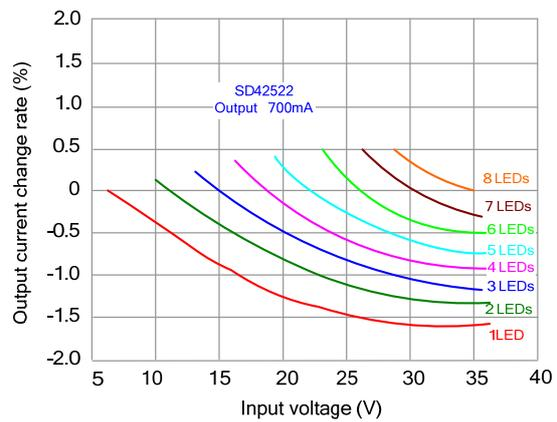
*Output 700mA current change rate following the input voltage*
