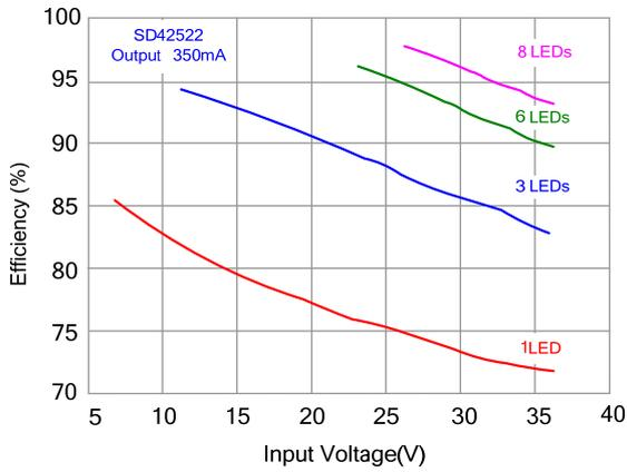
*Output 350mA efficiency changed following the input voltage*
